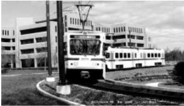
Light rail does not require a fully separated right-of-way because power is supplied by overhead catenary, rather than an electrified rail. It can operate on rights-of-way, which are fully or partially separated or at street level alongside traffic, as shown in these photographs from Baltimore (left) and Pittsburgh (right).
