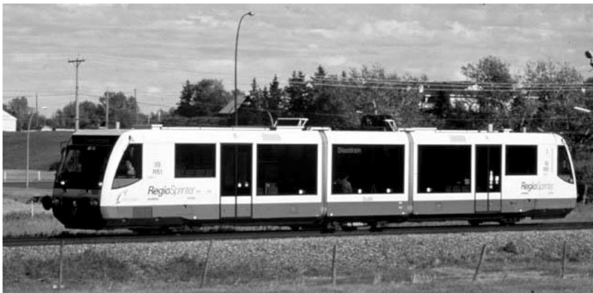
A number of medium-sized metropolitan areas, including Dane County, are considering newer lightweight, self-propelled diesel rail vehicles, such as the Siemens RegioSprinter shown here. These “hybrid” rail vehicles are said to be more economical than conventional commuter rail for purposes of lower-density suburban service. They can also stop and restart quickly enough to provide service between closely spaced stations within a city.
